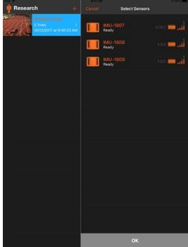
The signal bars show the signal strength of the sensor, and will be full if the sensor is very close. This can be used to identify sensors when many are discovered.
